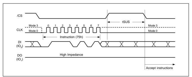
Figure 42a. Erase/Program Suspend Instruction (SPI Mode)
