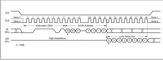
Figure 61a. Read Block Lock Instruction (SPI Mode)
