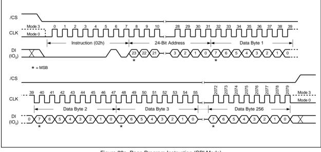
Figure 32a. Page Program Instruction (SPI Mode) 32-Bit Address is required when the device is operating in 4-Byte Address Mode
