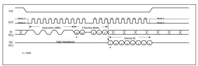
Figure 45c Device ID Instruction (SPI Mode)
