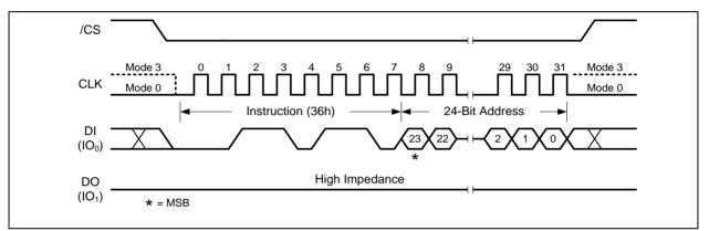
Figure 59a. Individual Block/Sector Lock Instruction (SPI Mode)
