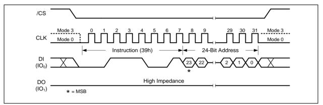
Figure 60a. Individual Block Unlock Instruction (SPI Mode)
