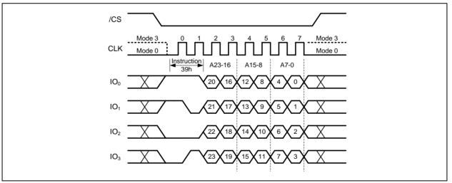
Figure 60b. Individual Block Unlock Instruction (QPI Mode)
