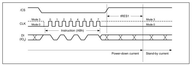
Figure 45a. Release Power-down Instruction (SPI Mode)
