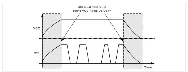
Figure 65b. Power-up, Power-Down Requirement
