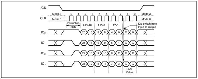
Figure 61b. Read Block Lock Instruction (QPI Mode)
