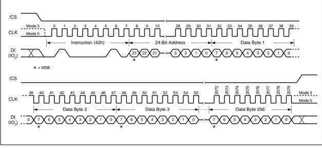
Figure 53. Program Security Registers Instruction (SPI Mode only) 32-Bit Address is required when the device is operating in 4-Byte Address Mode
