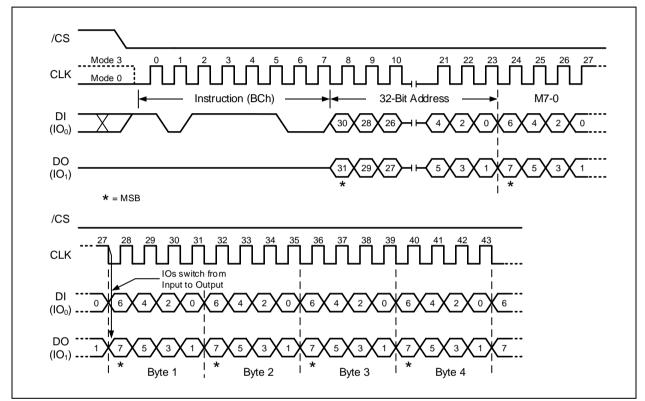
Figure 25a. Fast Read Dual I/O w/ 4-Byte Addr. (Initial instruction or previous M5-4+10, SPI Mode only)
