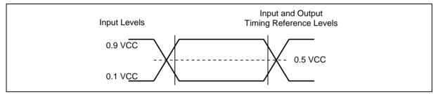
Figure 66. AC Measurement I/O Waveform
