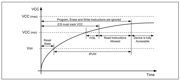
Figure 65a. Power-up Timing and Voltage Levels
