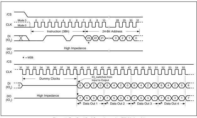
Figure 19. Fast Read Dual Output Instruction (SPI Mode only)
