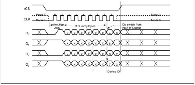
Figure 45d. Device ID Instruction (QPI Mode)
