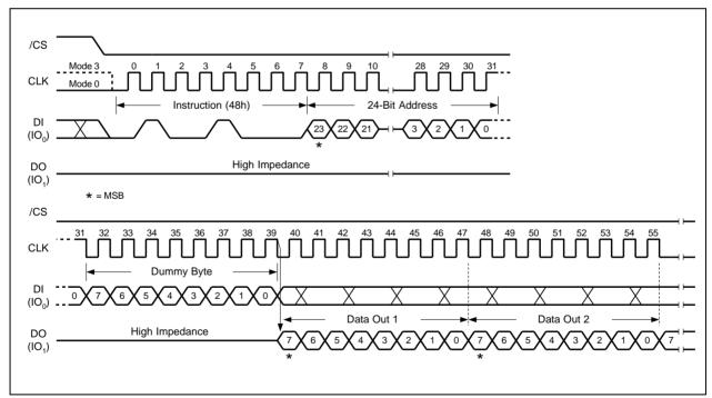
Figure 54. Read Security Registers Instruction (SPI Mode only)
