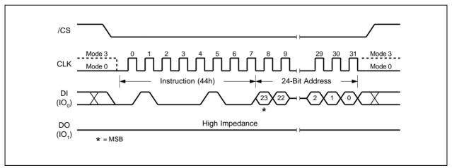
Figure 52. Erase Security Registers Instruction (SPI Mode only)
