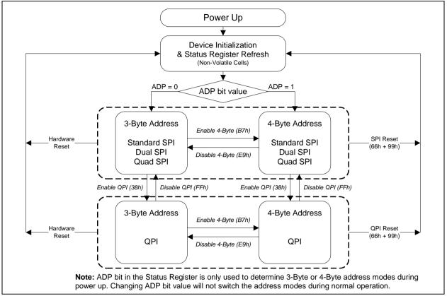
Figure 3. W25Q02NW Serial Flash Memory Operation Diagram
